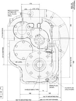
The maximum fore and aft installation angle permissible at rest is 17°.
